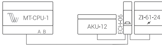
An example of 9÷30 V DC receiver power supply system
